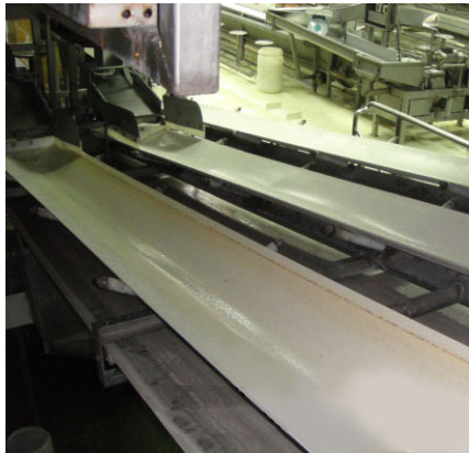
ESPOT 20CC Inclined conveying in pineapple processing.
