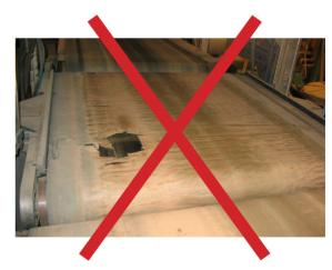
All these problems mean deteriorated belts have to be replaced often, hampering productivity (down time), while increasing maintenance costs.
