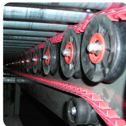
PowerMax V-Belt Idlers used with POWERWIST Roller Drive on a Live Roller Conveyor.
