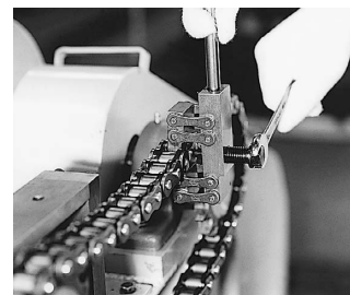
Fig. 5 How to cut a chain using a chain screw
