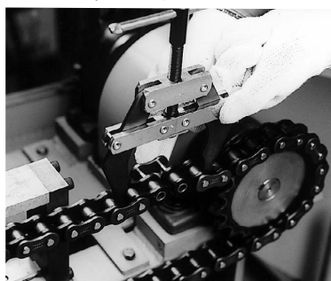
Fig. 9 Connecting between shafts
