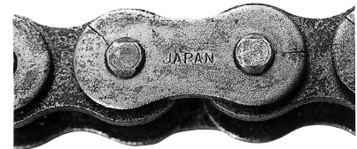
Fig. 32 Hydrogen embrittlement cracking
