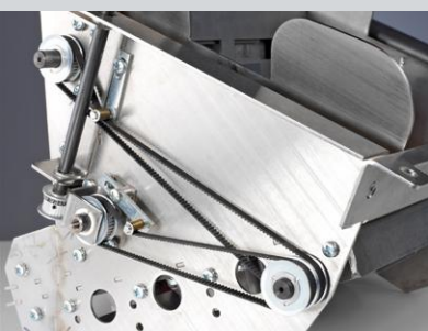
Drive unit of a friction feeder
