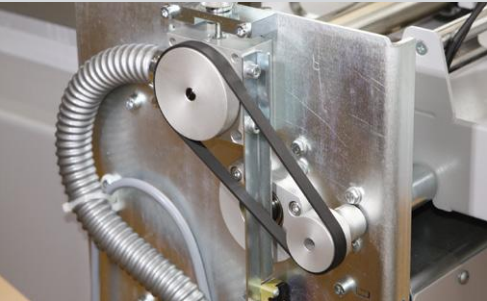
Light power transmission of paper drive axe
