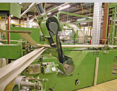
Tube winder belt 565 TW, 3150x120x4.0 mm
