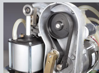
Flat belt drive of a suction pump
