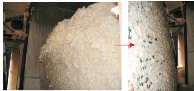
Inside the silo full of wool. The apron belt moves towards the silo.
