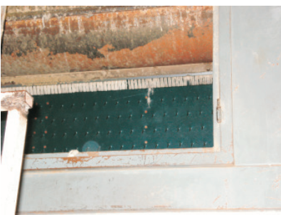
Expulsion roller at the top of the apron belt.
