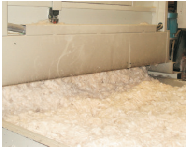
Wool exit, once mixed with bleaching additives.
