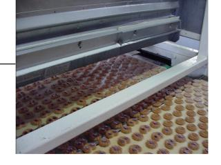
**POLER 08EFWP** belts are now being used. These belts have been on 9 to 12 months and still look good. As well as having great resistance to cracking, the belt coating gives better release and resists the sticky sugar build up.
