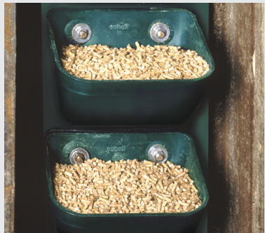
Buckets fitted to a belt conveying fodder.
